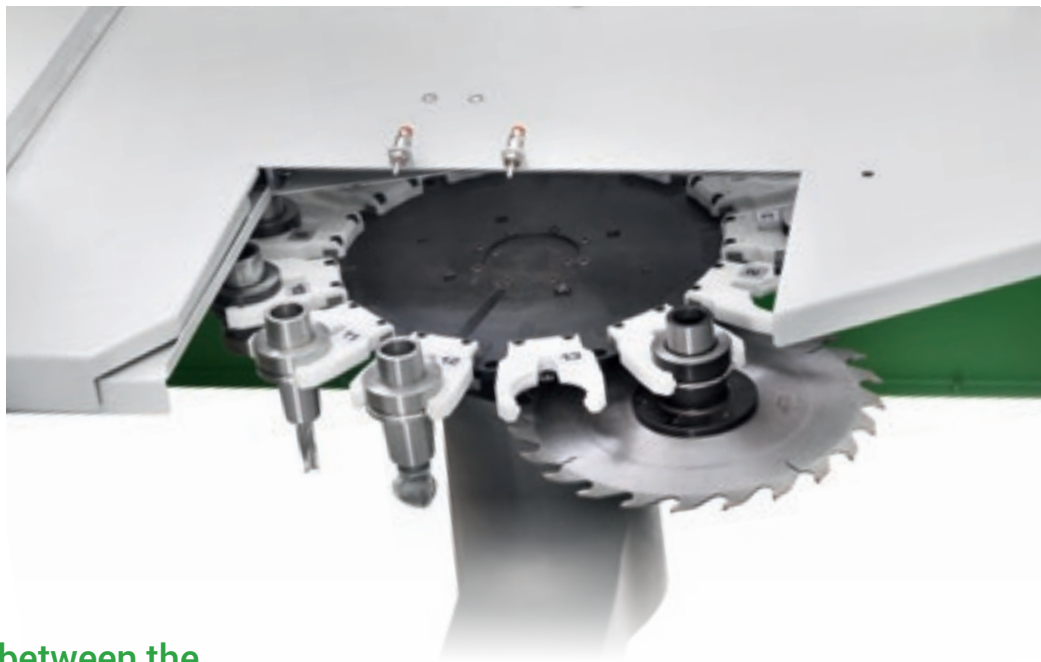
Rack tool magazine with 12 or 23 places, with integrated pick-up.
