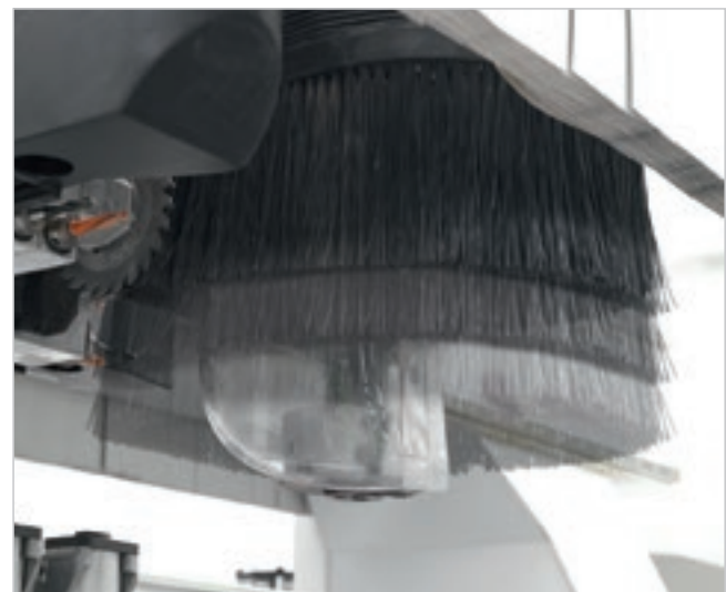
Adjustable suction hood with 6 settings (for 4 axes) and 13 setting (for 5 axes).
